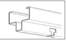
The profile can be suspended by appropriate bracket and hangers with regulation spring as per standard ceiling, and any panel is removable without to interfere with other panels.
