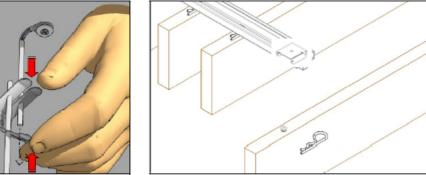
The system includes special cotter pins for panel anti-fall safety.
