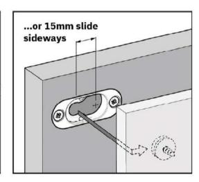
The Type 1 Flush Fix fits an oval rebate measuring  $22 \times 56 \times 8.1$ mm deep. It can also be used surface-mounted, creating an 8mm gap between the panels. Engage the Buttons in the Fix and slide the panel down by 15mm, until Button-fix goes 'click'. The Type 1 Flush Button-fix can be configured for sideways assembly too.
