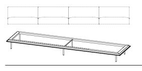
Structural sofa frame made of extruded aluminum profile with 6 legs made of steel rod. The legs can be assembled in different positions.
