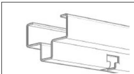
The profile can be suspended by appropriate bracket and hangers with regulation spring as per standard ceiling, and any panel is removable without to interfere with other panels.
