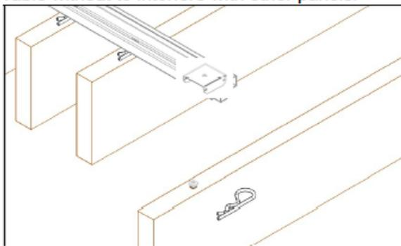
The system includes special cotter pins for panel anti-fall safety.
