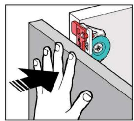
The Type 2 Fix is mounted to the back of the removable panel and the Type 2 Button to the side panel or supporting frame. The Fix Marker accessory makes sure the Button and Fix are correctly aligned.
